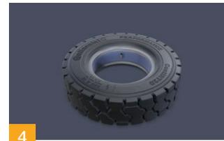
4 Working around the tire, press the TSR fully into position by pushing the TSR wings into the tire. It is very important to ensure that the TSR lies symmetrically inside the tire.
