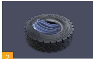
2 Fold the TSR in half to create a figure '8', and insert one loop into tire as far as possible.
