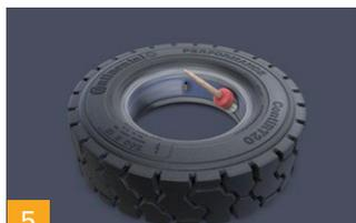
5 When the TSR is positioned in the tire, lubricate the visible surface of the TSR and the bead area.
