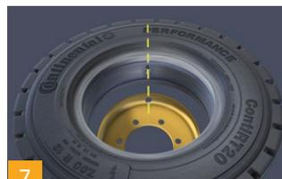
7 Align rim that valve slot is in line with TSR valve as shown, and let tire fall into position, whilst ensuring that valve remains centered in the slot.
