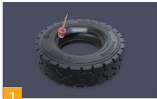
1 Lubricate bead area of the tire as well as the tire interior up to the middle of sidewall.
