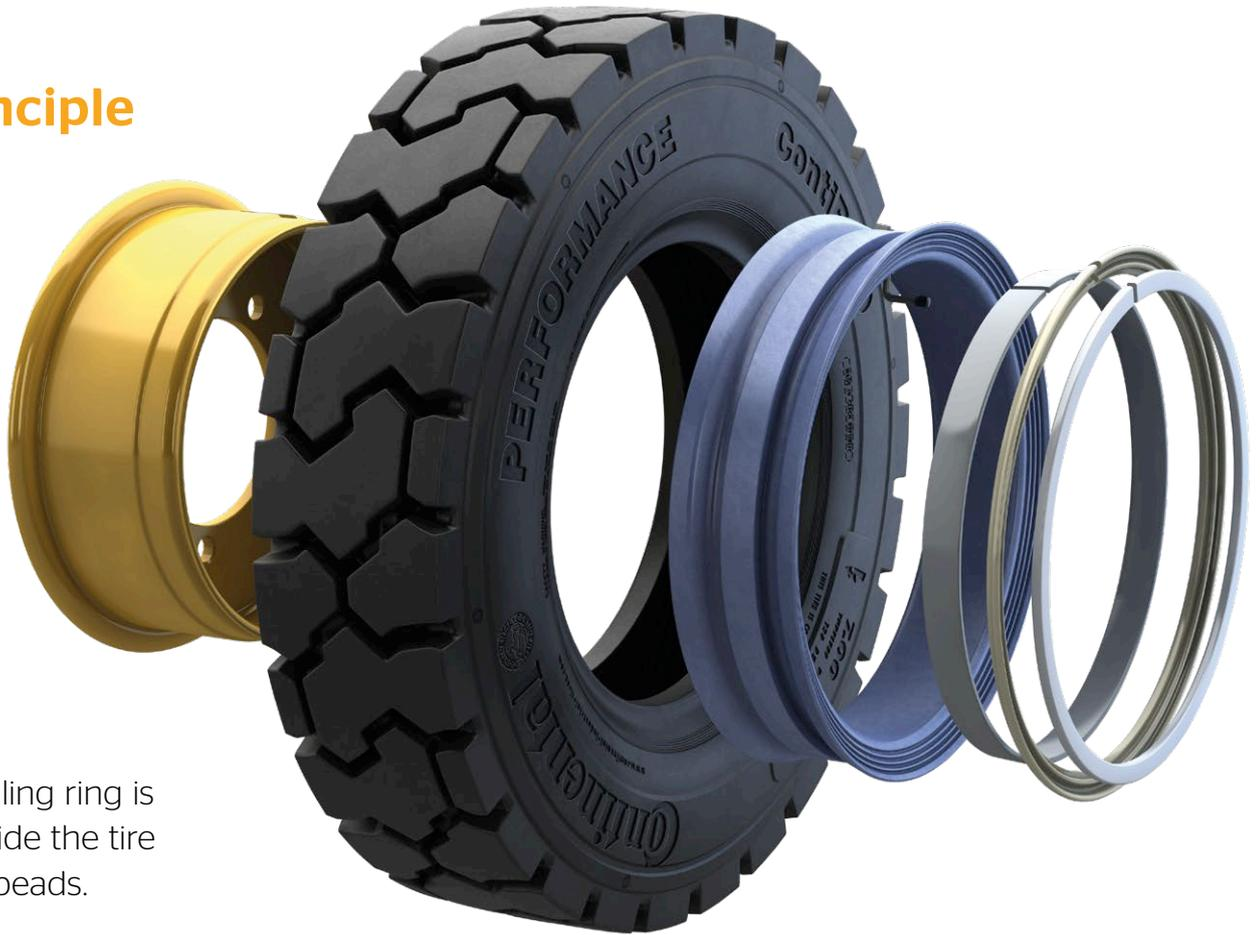
A rubber sealing ring is mounted inside the tire between its beads.
