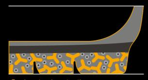
> Two-layer tread construction: combines high mileage performance in the cap compound with significant rolling resistance improvements in the base compound
