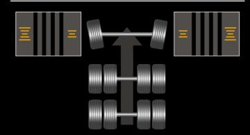
The inner shoulders wear more than the outer shoulders when front axle tires point outwards.
