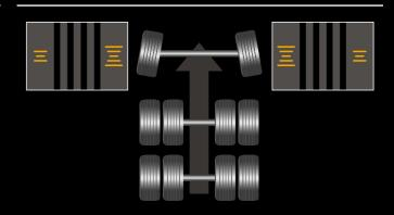
When wheels are correctly aligned tires wear evenly on both sides
