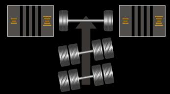
If the axles are not running parallel to one another the vehicle pulls to the side. As a result of counter-steering the tires wear more on one side.
