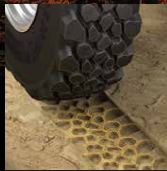
Special tread design with multiple block geometries
