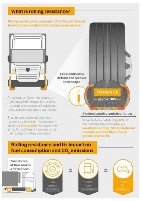
Chart showing the impact of rolling resistance as one of the key factors in saving fuel and cutting fleet operating costs efficiently.
