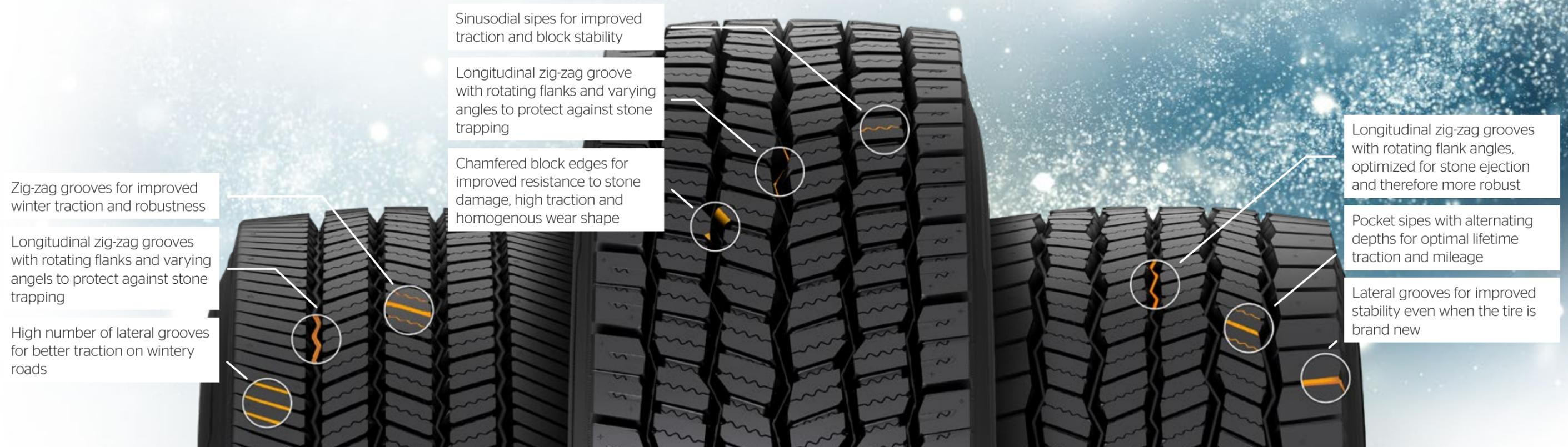
Sinusoidal sipes for improved traction and block stability
