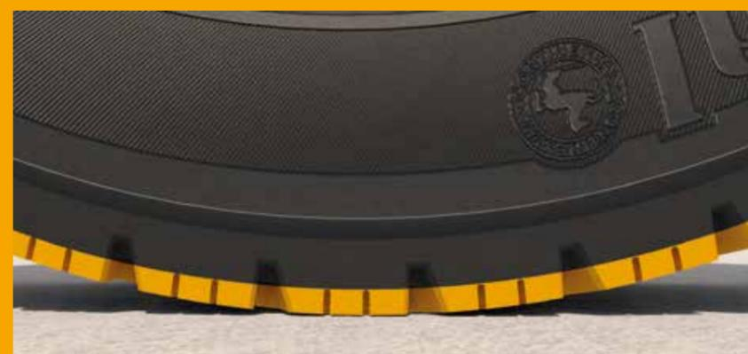
The Continental two-phase tread is like having two tyres in one: The tread structure changes from a more open structure for safer grip to a closed tread, which is optimised for low rolling resistance with equally good adhesion to the road surface. Once the winter tread has worn away, you are left with a steer and trailer tyre with very good consumption figures for the summer season.
