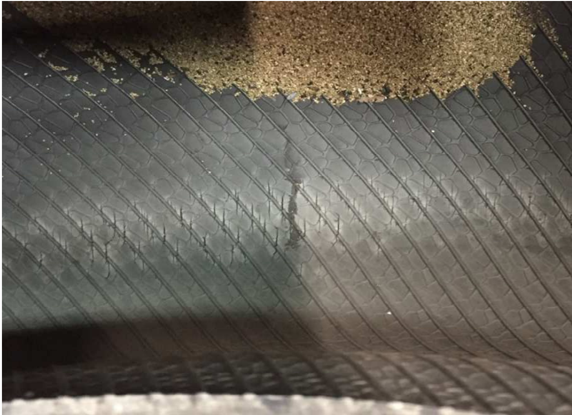
Fig1: Innerliner cracks caused by the balancing powder
