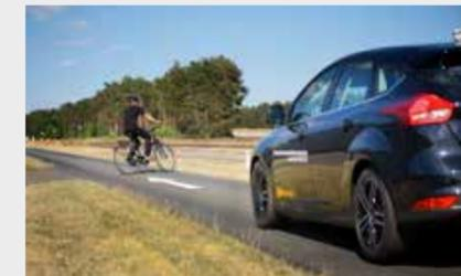
A demo car equipped with a radar sensor and a camera detects when a cyclist crosses the lane and warns when the object is in the path of the vehicle.
