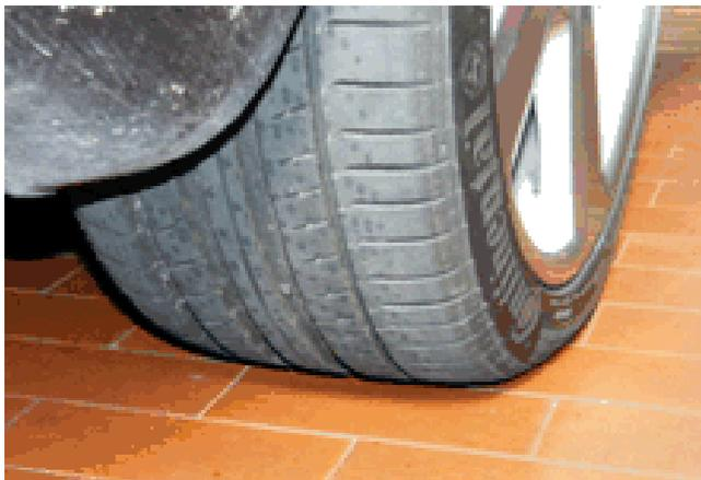
In operation, flat spotting may create a vehicle vibration due to the tyre being “out of round” (radial run out). Depending on the type of flat spot, the vibration normally disappears after a short driving distance as the flat spot is driven out.
