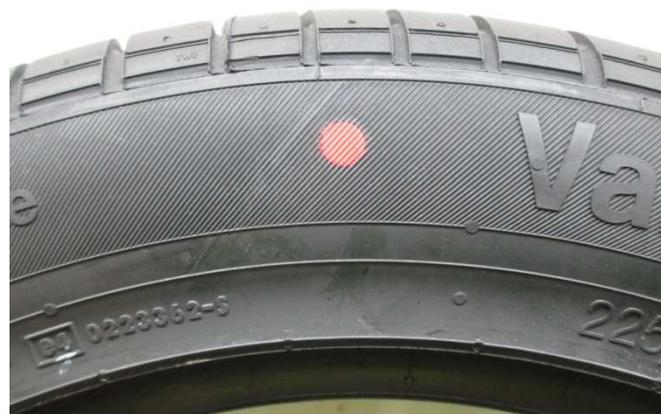
Some wheels (especially steel) have a low point dimple mark, if this is clearly shown then it is recommended to fit the tyre with the red dot aligned to this mark. This is the most accurate method of harmonising the tyre to the wheel.
