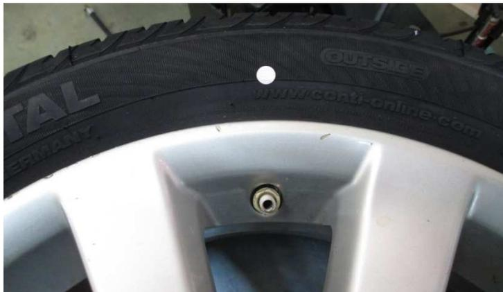
These markings are used to enhance the uniformity of the wheel assembly to improve the vehicles ride quality however they may only be relevant during the OE fitting process.
