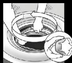
Working around the tire, press the TSR fully into position by pushing the TSR wings into the tire. It is very important to ensure that the TSR lies symmetrically inside the tire.
