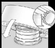
Align rim such that valve slot is in line with TSR valve as shown, and let tire fall into position, whilst ensuring that valve remains centered in the slot.
